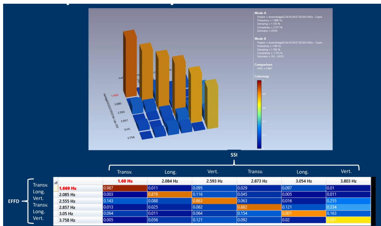
Figure 5: Compilation of vibration modes calculated with EFDD and SSI-UPCX methods
