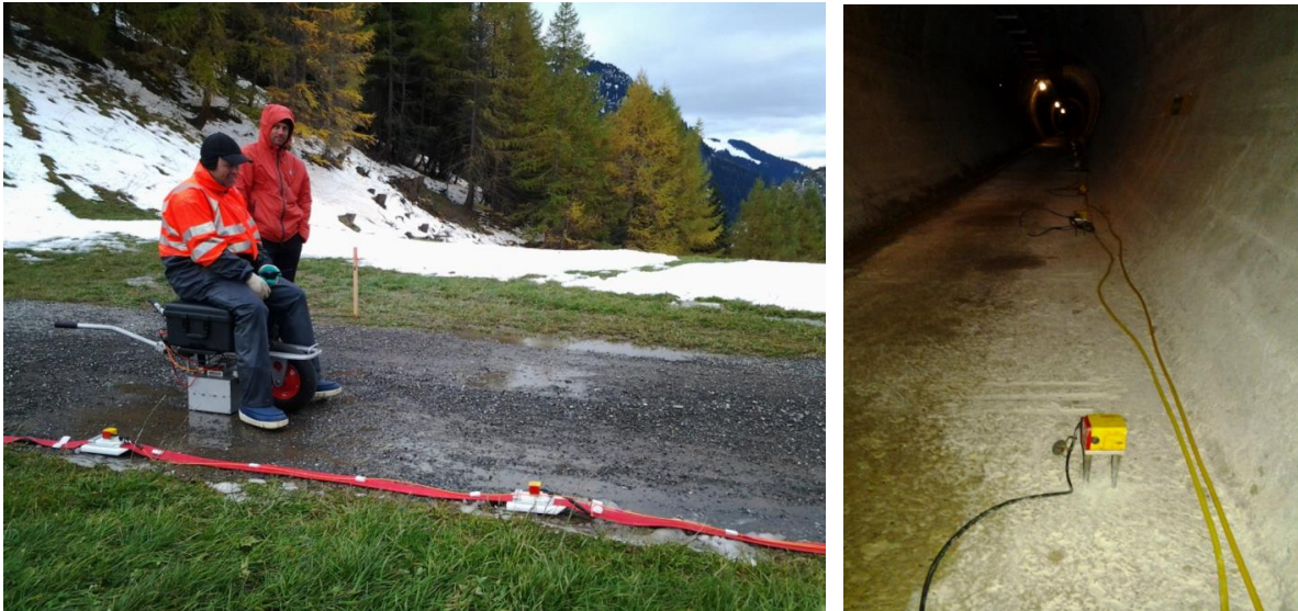
Figure 4: Seismic geophysical measurements, left: excitation of shear waves on the dam crest with shaker and part of geophone array mounted on a landstreamer system; right: geophone array in the inspection gallery in the inner dam body [3]
